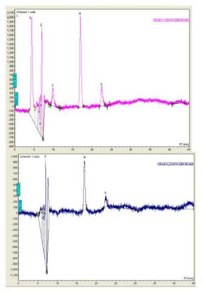
At absorption maxima of 284 nm, fluid A shows 5 peaks while fluid B shows 3 peaks, indicating the presence of additional entities in the suspect batch of peritoneal Liquid chromatography mass spectrometry analysis of normal (top) and suspect (bottom) dialysate batches.
